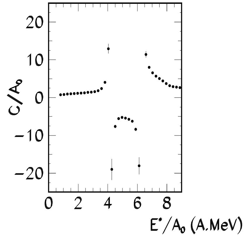
$$C_P = \frac{C_{\text{can.exp.}}^2}{C_{\text{can.exp.}} - \sigma^2 / T^2}$$
