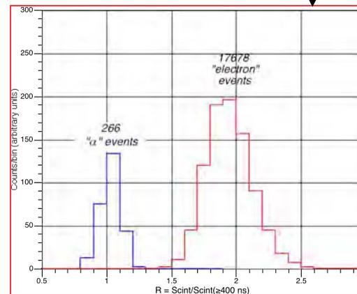
Experimental comparison of short/total electrons  $F_{prompt}$  for 2.3 litre chamber
